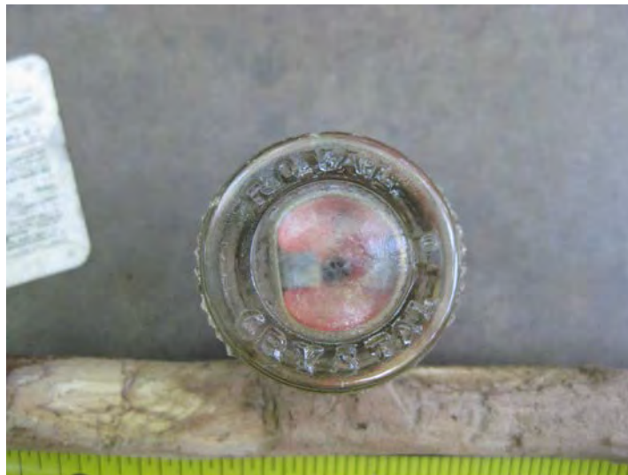
Figure 9. Close-up of Royal Crystal fuse, view down.
