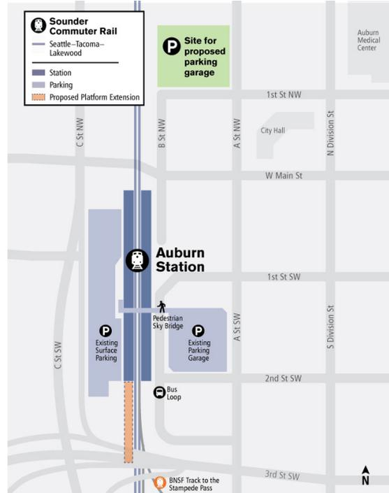
**Figure 4-7 Auburn Station Proposed Platform Extension**
