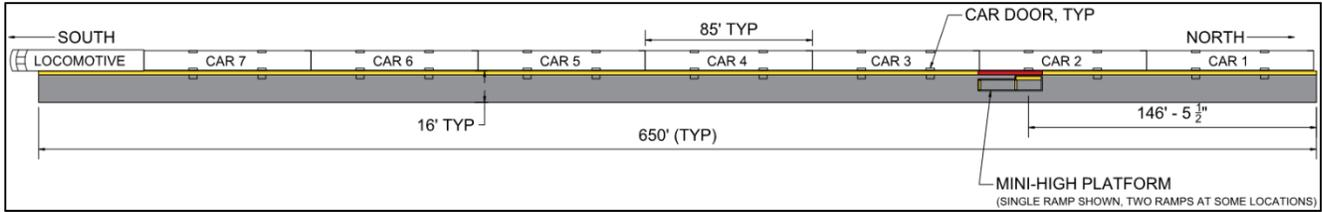
**Figure 4-12 Layout of a Typical Sounder South Train and Platform Today**
