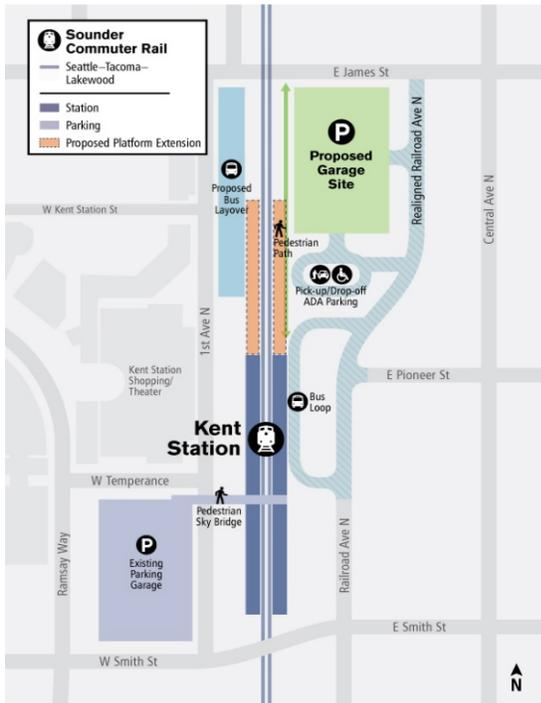
**Figure 4-8 Kent Station Proposed Platform Extension**
