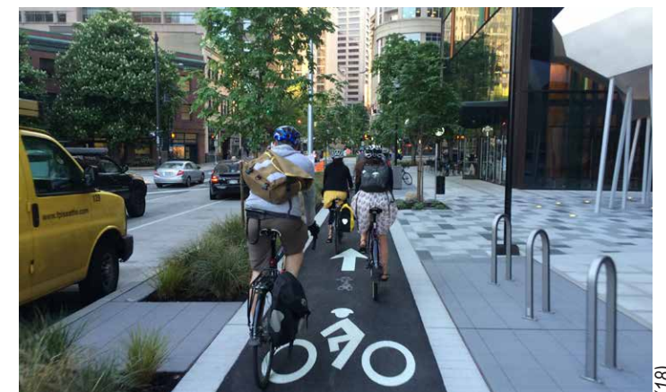
Landscaping and bike racks are used to separate cyclists from pedestrians in an adjacent sidewalk and plaza
