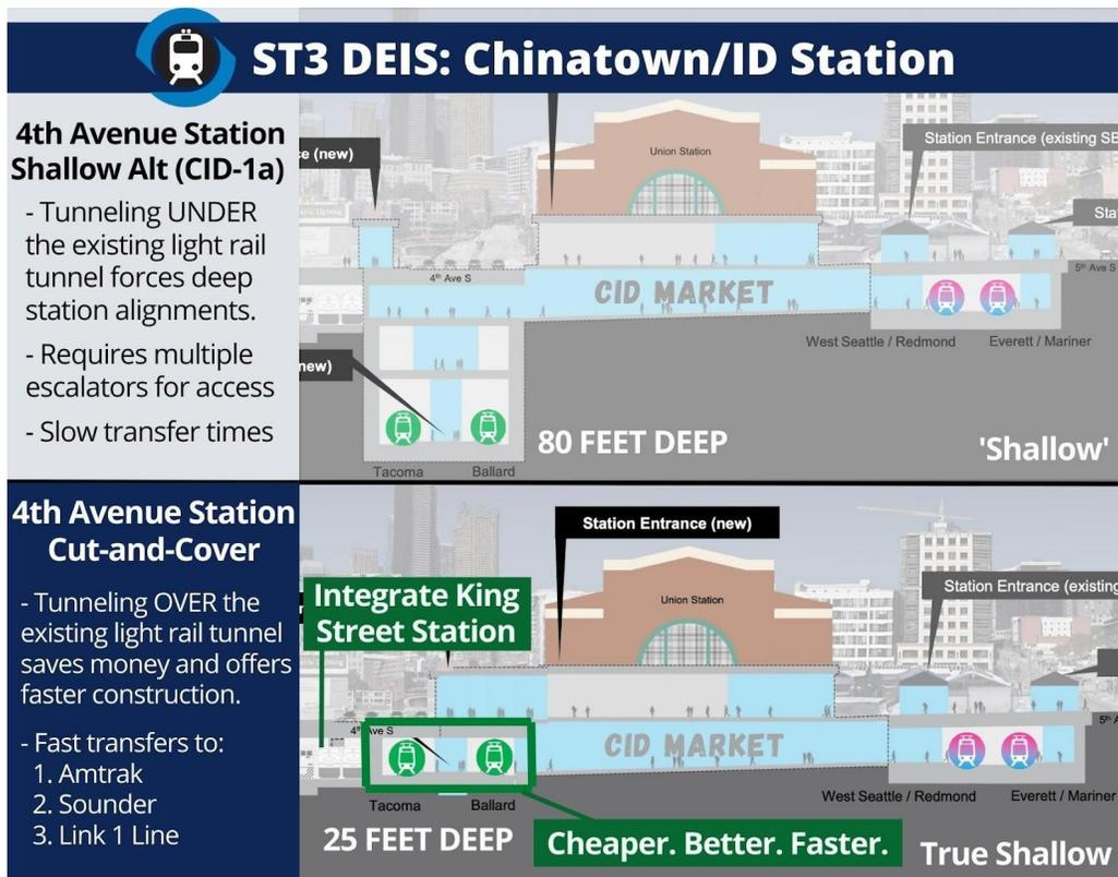
Going under the existing light rail tunnel is a major driver for the problematic tunnel depth we see for WSBLE in CID and Midtown. The solution is an opportunity to study a partial cut-and-cover option in conjunction with an improved 4th Ave viaduct rebuilt over the existing light rail tunnel. Fewer of the neighborhood’s housing units and businesses line 4th Ave
