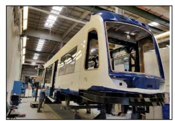
The second car undergoing paint inspection
