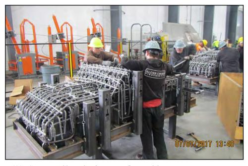
N180—Crews assembling rebar for pre-cast floating slab sections.
