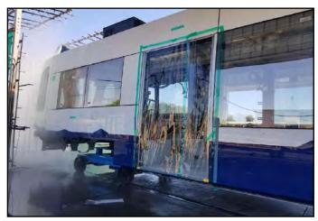
The first car undergoing water test.
