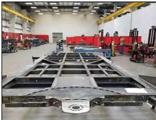
Underframe assembly for the carbody.
