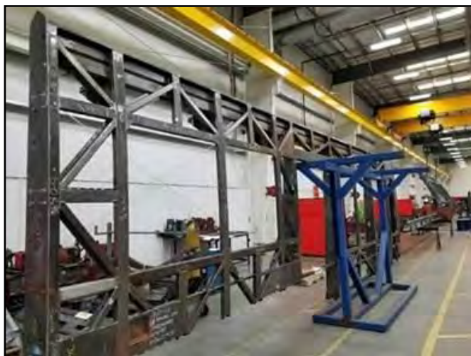
Side wall assemblies for the car body.
