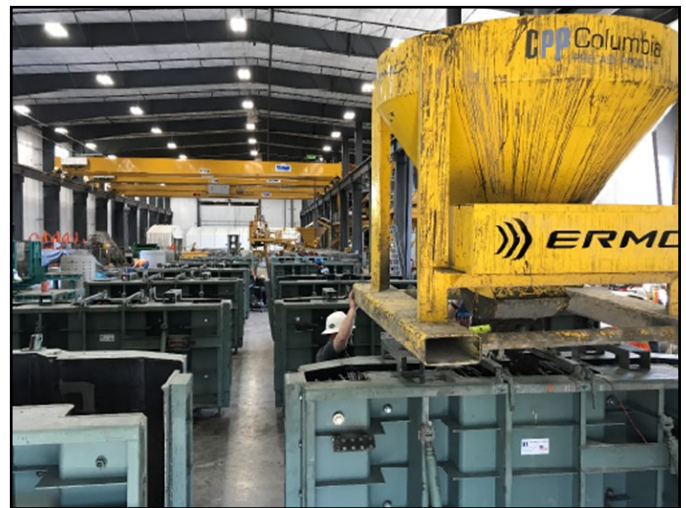
Columbia Precast: 3'-10" floating slab being cast.
