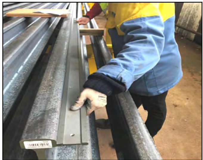
Verification of the rail-end straightness at British Steel Facility in Hayange, France.
