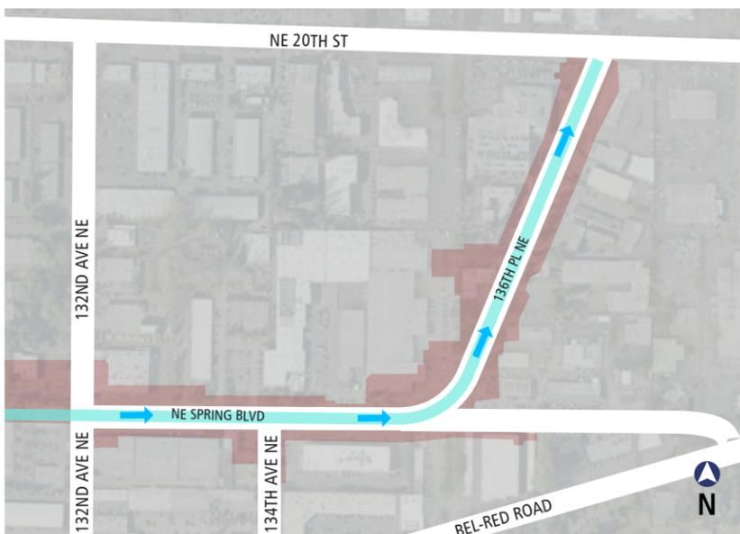
Construct light rail guideway in the center median along NE Spring Blvd and 136th Pl NE, including installation of new electrical Overhead Catenary System foundations and poles, track and intersection street treatments. (Fall/Winter 2020 - Fall/Winter 2021)
