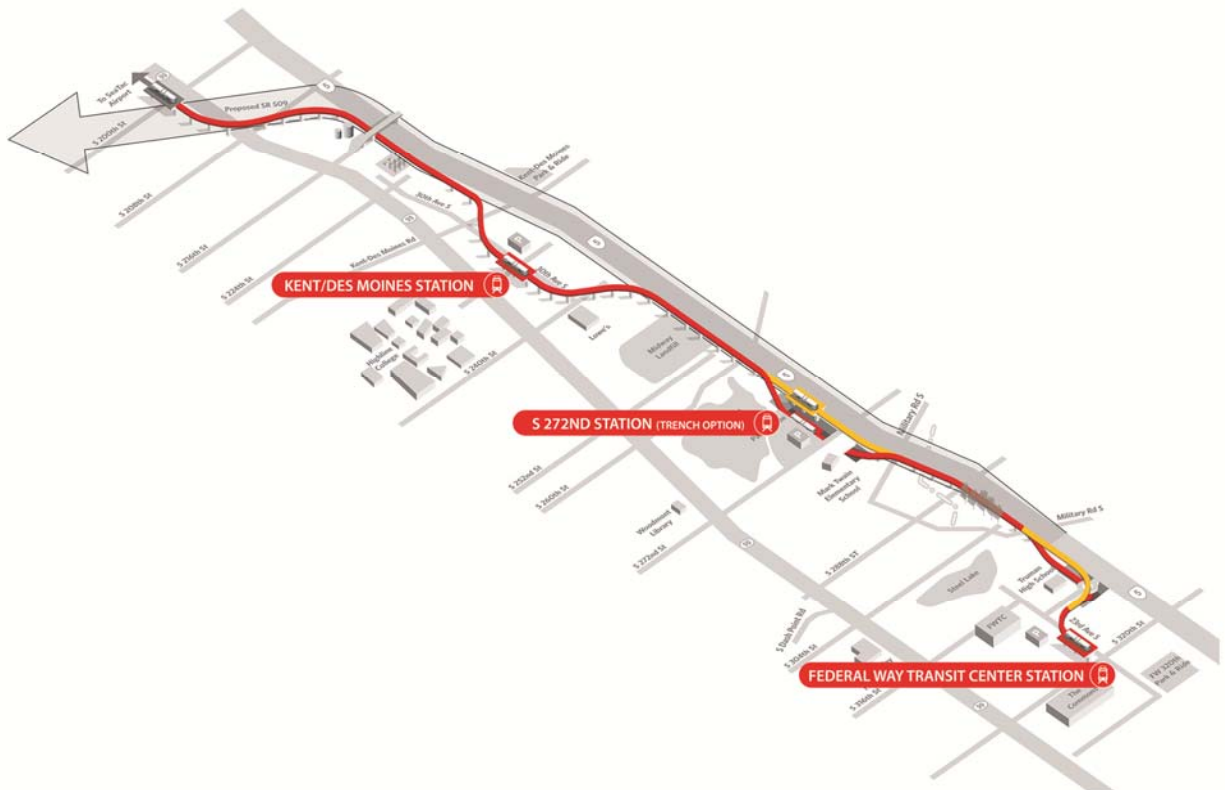
Figure 1 FWLE Preferred Alternative The red line represents the guideway with a trench station at S 272 nd and a trench guideway at S 317 th ; yellow represents elevated station and alignment options at these locations.
