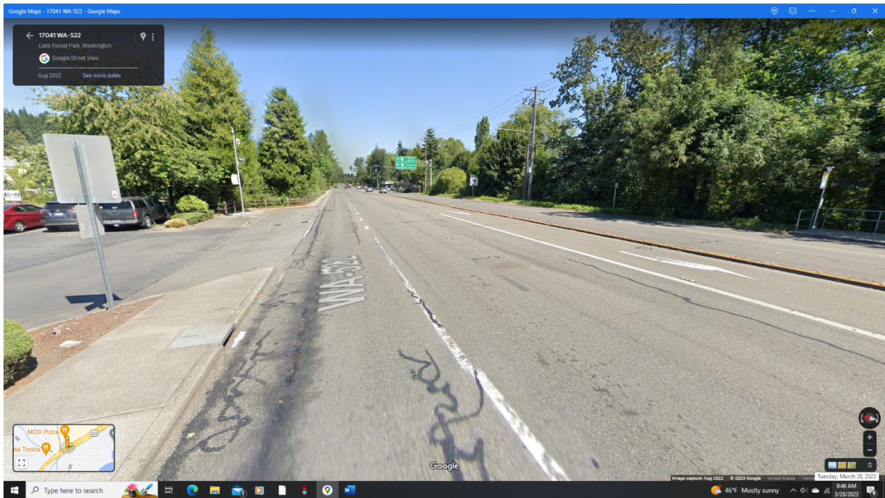
Figure 4 Existing section at Starbuck's approaching Ballinger Way. 77' curb-to-curb for 6 traffic lanes and a left-turn lane.
