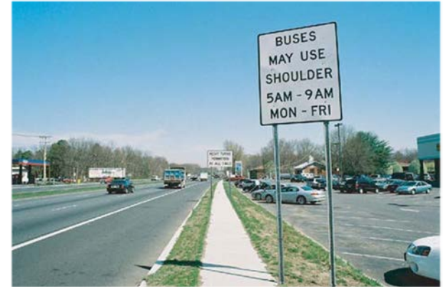
Static Bus-on-shoulder message sign on US 9 arterial in Old Bridge, New Jersey. (Source: TCRP Report 151)
