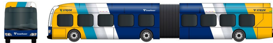
Articulated battery electric buses for shorter arterial route
