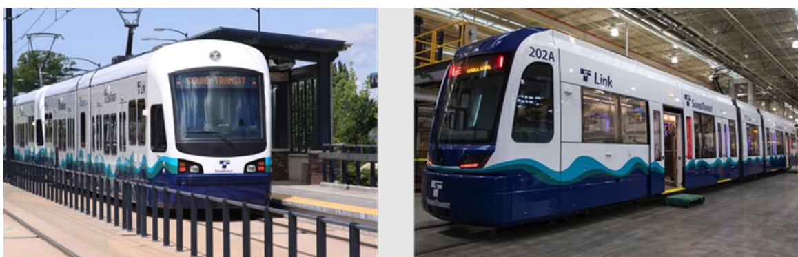
Figure 2. Sound Transit's Link light rail fleet includes Kinkisharyo Series 1 vehicles (left) and Siemens Series 2 vehicles (right).
